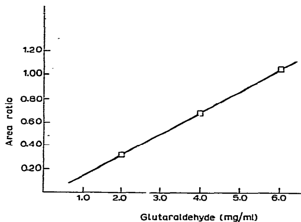
Fig. 2. Typical standard curve plotting peak area ratio of glutaraldehyde to internal standard vs. glutaraldehyde concentration (mg/ml).
